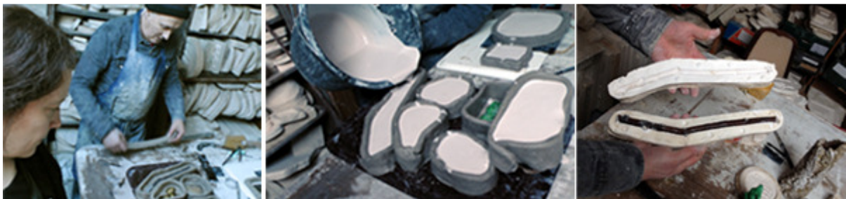
Above – the casting process, making the moulds, pouring in the plaster and a two part mould when dry and separated. 2015
