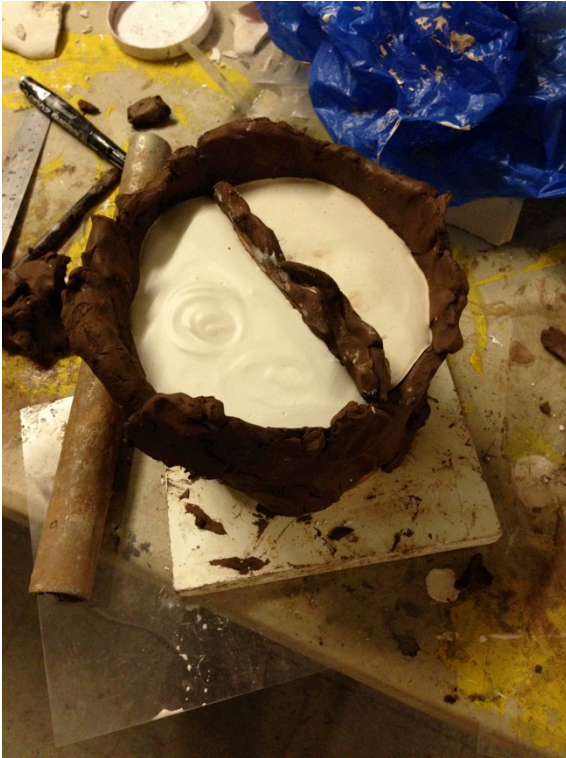
L to R: Making a plaster mould for concrete casting, detail of resulting concrete object, plaster cast using plastic cups
